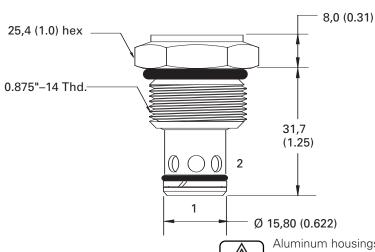
Aluminum housings can be used for pressures up to 210 bar (3000 psi) Steel housings must be used for operating pressures above 210 bar (3000 psi) Check valve
