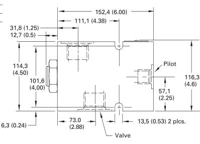
The POC1-10 is a pilot-toopen, screw-in cartridge type check valve.
