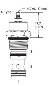
Dual Pilot Operated Check Valve Cartridge
