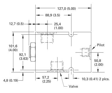
The SPC1-20 is an inline housing type, pilot-to-open check valve.
