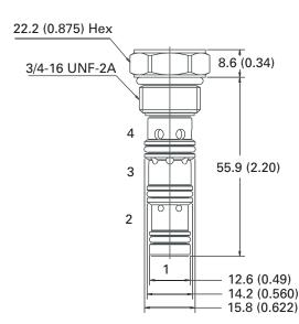
The DPC1-10 is an inline housing type, double pilot operated check valve.
