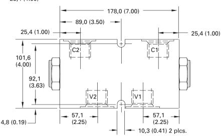
The DPC1-20 is an inline housing type, double pilot operated check valve.
