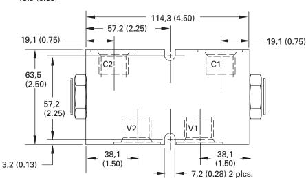
The DPC11-12 is an inline housing type, double pilot operated check valve.
