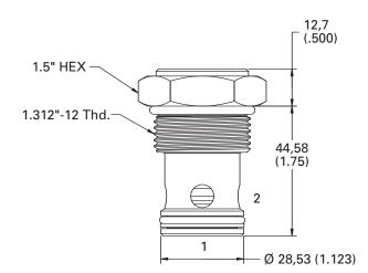
The RCV3-10-P is a poppet type, screw-in cartridge check valve with stroke limiter.
