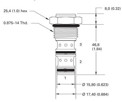
The SPC1-10 is an in-line housing type, pilot-to-open check valve.
